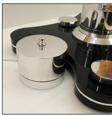
Place the drive belt over the engine pulley and the belt groove on the TMD bearing. The belt should
